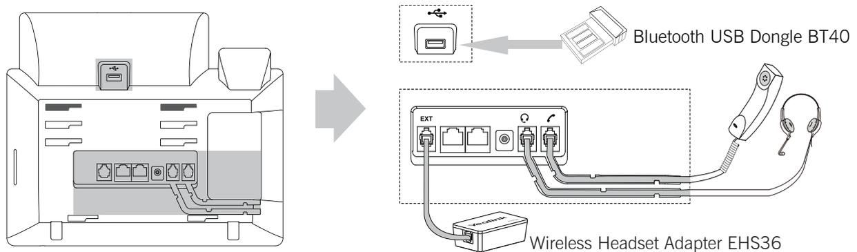
Note: The headset, Bluetooth USB dongle BT40 and wireless headset adapter EHS36 should be purchased separately. The EXT port can also be used to connect the expansion module EXP40.
